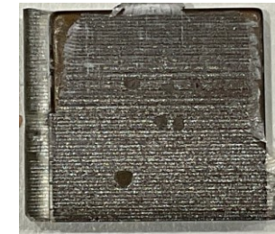
Phosphating coating with much attached adhesive
