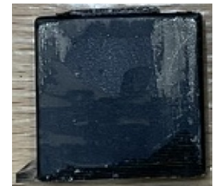
Epoxy coating, partially scratched off
