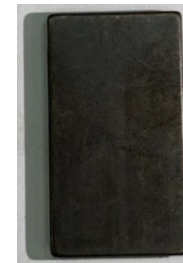
Phosphating coating without adhesive attached
